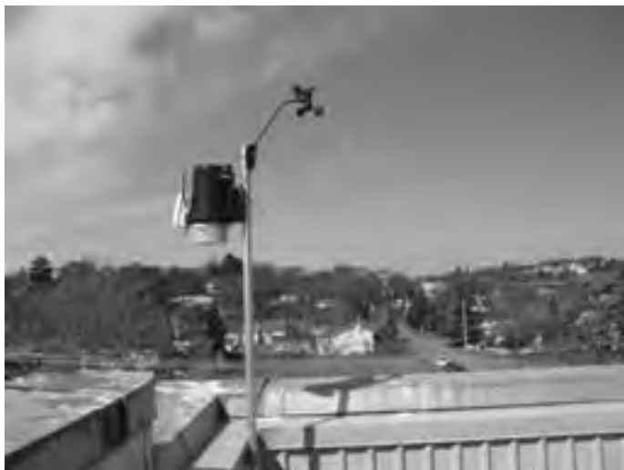
Figure 2. Photograph of the Davis Vantage Pro2 Plus weather station installed on top of Oaklands Elementary school in Greater Victoria School District 61.
